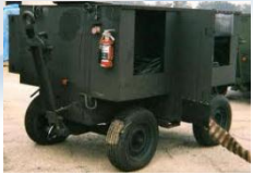
Aviation Ground Power Unit
